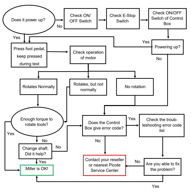
Write down the Error Code flashing in the screen of Control Box if needed to contact the Picote Service Centre. The Error Code narrows down the list of possible problems with your Miller unit.
