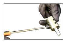
Feed the shaft through the socket to the end and **securely fasten**. The outer casing should reach all the way to the base of the shaft socket to protect the shaft.
