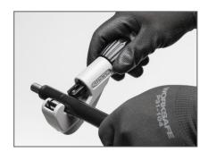
Always inspect the outer casing before each use. Easiest and safest way to shorten the outer casing to the correct length is using sheath cutter. Only the needed amount of bare shaft should be exposed in all times.
