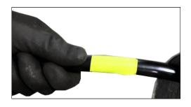
Attach a visual marker (tape) to the outer casing of the flexible shaft. Place it around half a meter from the end point of the shaft. The mark will indicate the tools location and prevent possible injuries when the tool is removed from the pipe, including injury by rotating parts.
