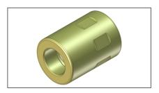
Always use a Sleeve Bearing for thin outer casing when using Super Midi Miller. It prolongs the lifetime of the flexible shaft and prevents the outer casing from melting in the tool end. Sleeve bearings can be re-used when outer casing is shortened.
