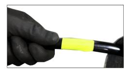
Attach a visual marker (tape) to the outer casing of the flexible shaft. Place it around half a meter from the end point of the shaft. The mark will indicate the tools location and prevent possible injuries when the tool is removed from the pipe, including injury by rotating parts.
