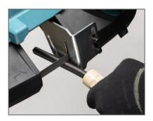
Always inspect the flexible shaft before each use. If there are potential weak points or the shaft is damaged, cut off the damaged length using a band saw.
