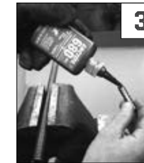
3. Apply Loctite Retaining Compound to splice core.
