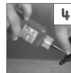
4. Apply Loctite Retaining Compound to the end fitting.
