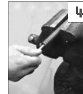
4. Insert splice core into cable one turn.
