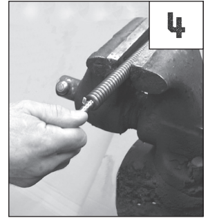
4. Insert splice core into cable one turn.
