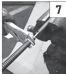
7. Place vise grips on free cable end and turn counterclockwise.
