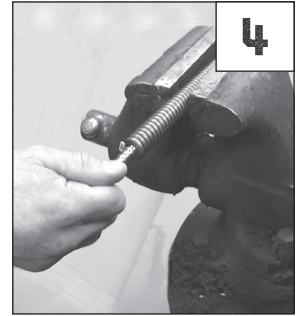
4. Insert splice core into cable one turn.
