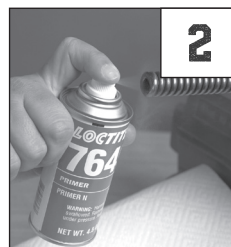
2. Spray Loctite Primer in and around the cable end to thoroughly remove grease and grime.
