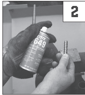
2. Spray Loctite Primer in and around the cable end and splice core to thoroughly remove grease and grime.
