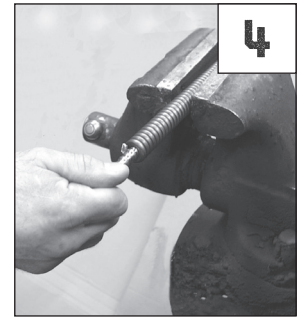
4. Insert splice core into cable end one turn.
