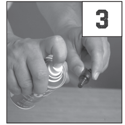
3. Spray Loctite Primer on the end fitting to thoroughly remove grease and grime.
