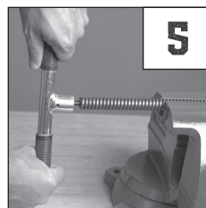
5. Using the wrench (part number EW), screw the fitting into the cable end until fitting is totally sealed.
